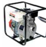
WX/WB 1" to 4" centrifugals Honda up to 1800 LPM & 40 MTRS
