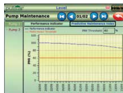
Screenshots showing the Predictive Maintenance Index curves drawn by the Ultimate Controller
